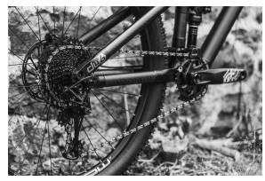
Fasten the dérailleur to the hanger, ensuring that the B-tension is seated correctly. Reconnect the chain using the provided power link. The chain is already cut to size and gears indexed.
