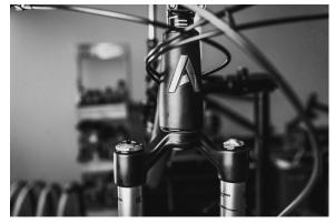
Install the forks into the headset, attaching the stem to the steerer tube. Preload the top cap and tighten the clamp bolts (ensuring that the stem is aligned correctly).
