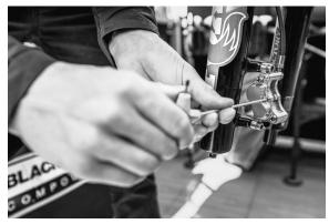
Fasten the controls to the handle bars. positioning as desired. Using a T25 torx key, attach the brake rotors to the hubs. Progressively tighten the bolts in a star sequence until torqued to 6.2Nm.
